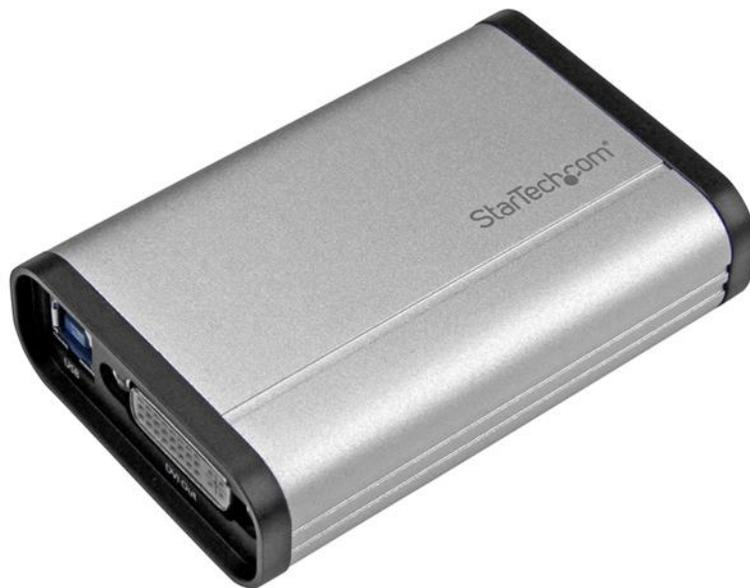
This capture device turns your USB 3.0 computer into a digital video recorder for high-quality DVI video, leveraging USB 3.0 transfer speed to capture raw 1080p video at 60 frames per second. The capture device records video from your DVI source device and also includes a 3.5 mm audio input jack that lets you record the video's accompanying analog audio output, or add your own independent audio source for voice over commentary.
