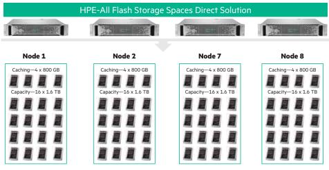
Figure 1. HPE All-Flash Storage Spaces Direct Solution
