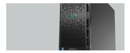
Their HPE ProLiant ML350 Gen9 server has dual power supplies and other redundancy features, which are very important to the firm. Plus, it comes standard with the latest Intel Xeon processors, HPE DDR4 SmartMemory, and support for up to 48 small form factor (SFF) drives. The firm uses 10K RPM SAS drives, configured in a RAID 5 array.
