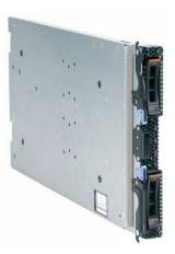
The BladeCenter® HS23E offers you flexible configuration options and provides you the energy efficiency and density you need. Combine the twelve DIMM slots supporting up to 192 GB of DDR3 memory at 1600 MHz, with the integrated 1 Gigabit Ethernet (GbE) onboard for flexibility with value.
