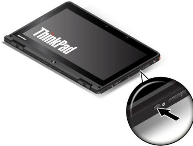
In tablet mode, the keyboard, the ThinkPad trackpad, and the TrackPoint pointing stick are automatically disabled.
