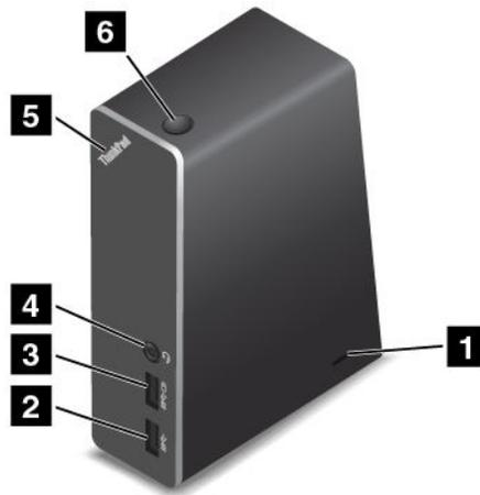
**1 Security-lock slot:** To protect your dock from theft, you can purchase a security cable lock, such as a Kensington-style cable lock, that fits this security-lock slot to lock your dock to a desk, table, or other non-permanent fixture.
