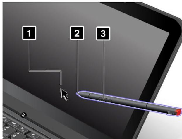
To make a selection (single click), tap the display once with the pen. To double-click, tap twice without pausing. To right-click, tap and hold the tip of the pen on the display for one second and then release the pen; or press and hold the click button **3** and tap the tip on the display.
