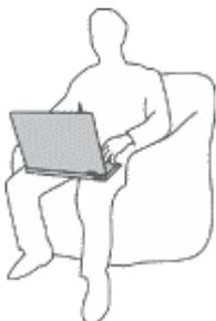
When your computer is turned on or the battery is charging, the base, the palm rest, and some other parts may become hot. The temperature they reach depends on the amount of system activity and the level of charge in the battery.
