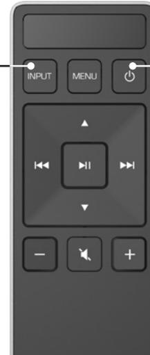
\* Auto detect function only occurs once when the Sound Bar is first powered on. To enable this feature again, you must do a Factory Reset (see the *Using Button Combinations* section for more information) or press and hold the INPUT button for 3 seconds.
