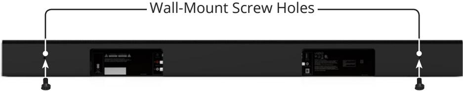
Insert the two wall-mount screws into the wall-mount screw holes, and then tighten them with a Phillips screwdriver.
