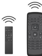
Point both the sound bar and TV remotes towards the front of the sound bar when programming.
