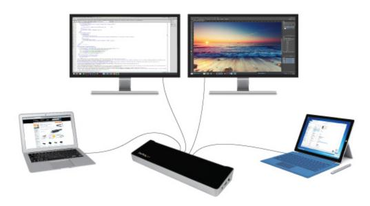
You can create a dual-monitor workstation that connects with two laptops if you have DisplayPort™ and HDMI® displays. Alternatively the dock supports a single 4K DP monitor, for 4K x 2K (3840 x 2160p - 30Hz) cinemaquality resolution and vivid picture quality.
