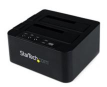
The SATDOCK22RE USB and eSATA Standalone Duplicator Dock lets you duplicate/clone an existing hard drive without the use of a host computer system, or can be connected to a computer system for use as an external hard drive dock.
