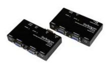
The ST122UTPA VGA Video Extender over Cat 5 with Audio allows up to 4 (2 local and 2 remote) monitors to be connected to a single PC. The video signal and corresponding audio are sent to the remote unit over standard 4 pair Category 5 or better (Cat 5e recommended) UTP cable, supporting extended video distances of up to 150m / 500ft.
