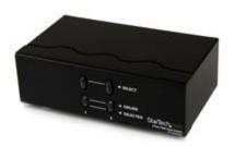
The ST122VGAU VGA Auto Switcher lets you share a display between two computers and prioritize your VGA signals. The VGA switch features a primary and secondary VGA input port, and automatically outputs the signal from the primary input. When the signal feed connected to the primary input port is cut, the switcher automatically defaults to the video signal on the secondary VGA input port.
