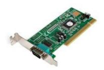
This 16550 Serial PCI Card can be installed in a computer PCI slot to add an RS232 serial port - a cost-effective solution for connecting any new serial device or old legacy serial device, with data transfer rates of up to 115.2 Kbps. The serial card features a low profile/half-height bracket, suitable for installation in low profile/small form factor computer cases.
