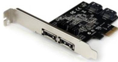
The PEXESAT322I PCI Express SATA III Controller Card (6 Gbps) gives you the option to add 2 internal or external SATA ports to your computer, through a single PCI Express (x1) card slot. The card features on board jumper selection, which enables you to configure the card to provide 2 internal or external SATA III ports, or one of each, as needed.
