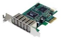
The PEXUSB7LP Low Profile PCIe USB 2.0 Adapter Card offers a cost-effective way to add seven USB 2.0 ports to a small form factor computer for enhanced versatility and performance.
