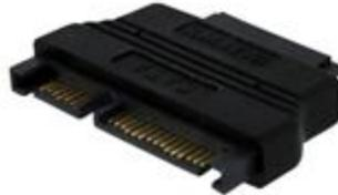
The SLSATAADAP Slimline SATA to SATA adapter is a cost-saving solution that allows you to connect a Slimline SATA optical drive to a standard SATA motherboard connection.
