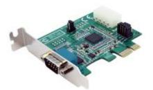
The PEX1S952LP 1 Port Low Profile Native PCI Express RS232 Serial Adapter Card with 16950 UART adds an RS232 (DB9) Serial Port with data rates up to 460 Kbps to a computer through an available low profile PCIe slot, while relying on a native, single-chip design (Oxford OXPCIe952) that harnesses the capability of true PCI Express - ensuring maximum performance and reliability and reducing the load applied to the CPU by as much as 48% over conventional (bridge chip) serial cards.
