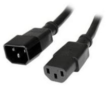
The PXT100 6ft PDU Style Computer Power Extension Cord features one C13 computer power (female) connector and one C14 hooded (male) power connector, and enables you to connect your server to a C13-equipped UPS or PDU.
