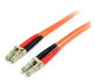
The FIBLCLC3 3-meter (10ft) Multimode 62.5/125 Duplex Fiber Patch Cable is terminated at both ends with LC (male) connectors, to provide the necessary connection between fiber networking devices for high-speed, long distance networks.
