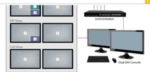
The KVM switch integrates front, push-button controls for simple switching between PCs, choosing your desired display mode and accessing the KVM menu, plus hot-keys and RS-232 command support, for flexible control.
