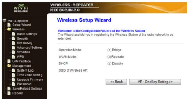
7. The Repeater will automatically pre-configure itself with default information and then reboot. If there are multiple wireless networks or a problem occurs with the automatic setup, Advanced Configuration may be required. Otherwise the setup is complete.
