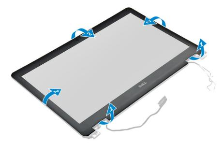
4 Remove the display bezel from the display assembly.
