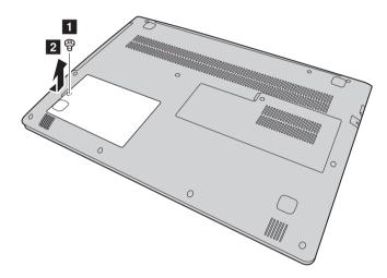
f A Remove the hard disk drive by gently pulling it in the direction of the arrow f B.
