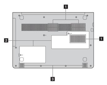
**1 Ventilation slots** Dissipate internal heat.
