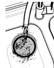
Tap the filter over a bin to remove any dirt/debris. Wash the filter under running water (40 degrees max).
