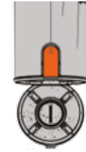
Hold dirt container over a bin, press the dirt release button to open, allow the dirt to fall out.
